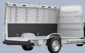
High-strength steel cage-type body structure
