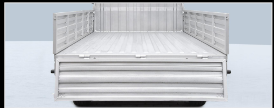
3.15m × 1.53m, oversized cargo box for increased hauling capacity.
