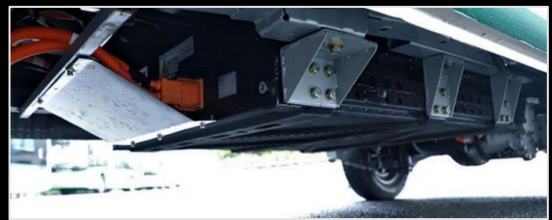
41.86 kWh CATL battery, efficient and safe.
